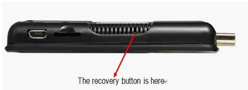
3. Don't loose the stick, at same time, insert the micro USB port to the unit USB OTG port, after 3-5s, loose the stick.
