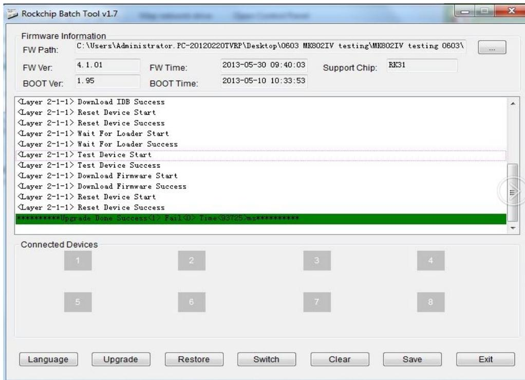
When this above prompt window appears, then means recovery is successful, pull out USB cable, total process is finished.
