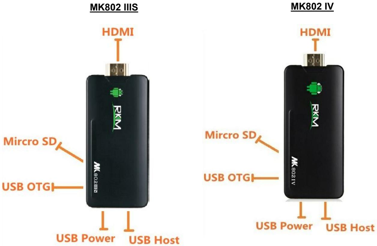
Micro-USB Power: Connect with TV USB/ USB power supply to power the device.
